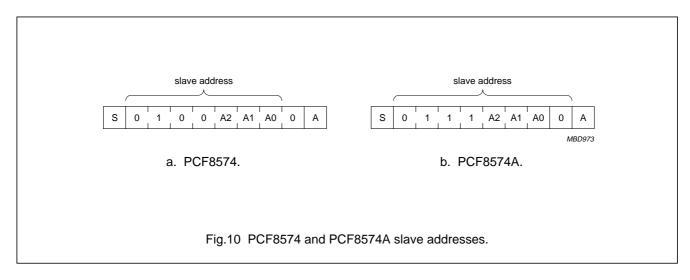
Each of the PCF8574's eight I/Os can be independently used as an input or output. Input data is transferred from the port to the microcontroller by the READ mode (see Fig.12). Output data is transmitted to the port by the WRITE mode (see Fig.11).
