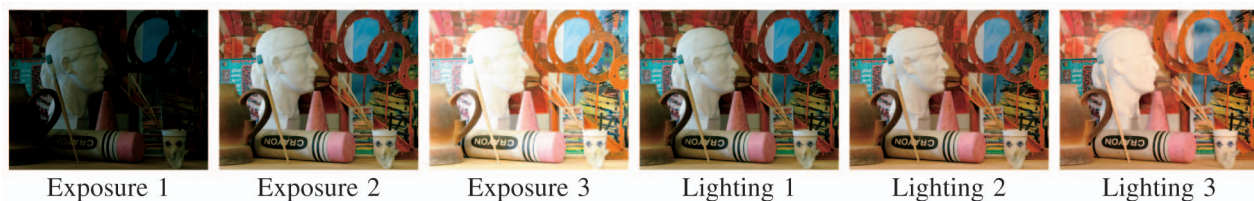
Fig. 12. The left image of the Art data set with three different exposures and under three different light conditions. The right images have been captured under the same conditions, such that 3 \times 3 combinations of matching are possible, separately for different exposures and light conditions. (a) Exposure 1. (b) Exposure 2. (c) Exposure 3. (d) Lighting 1. (e) Lighting 2. (f) Lighting 3.
