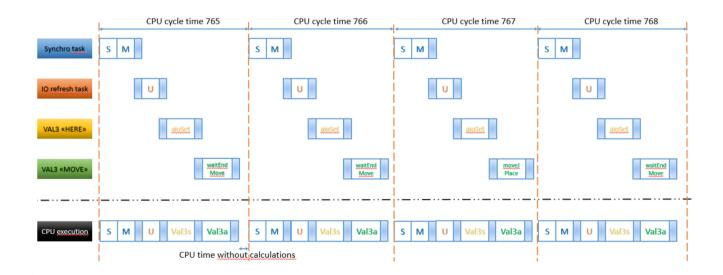
If we focus on the IO refresh, we see that the first aloset is after the first IO refresh task, it means that the coordinates collected in the cycle 1 by the synchro task are sent to the Fieldbus during the cycle 2:
