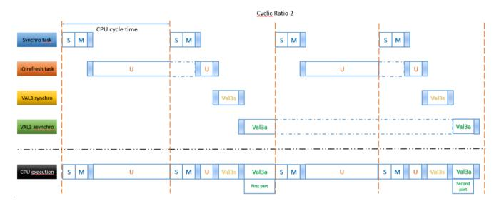
Obviously it is recommended to set this value as little as possible. In other words to increase this value only if it is needed. A bigger value of cyclicratio will lead to a bigger discrepancy between the Val3 program and the IO refresh.
