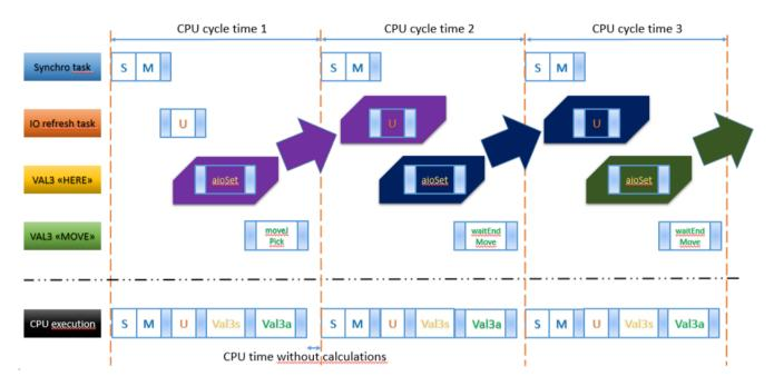
It means that if we are working with a cycletime of 4ms, the position sent on the fieldbus has a delay of 4ms compared to the position measured. Here is clear that if we use an asynchronous task to send the position to the fieldbus we are not sure of the frequency of the refresh rate of the IOs
